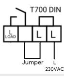
For 24V (or other low voltage) relay operation voltage connect a power supply with the wanted voltage through two lower left connection screws on the bottom connector (see picture). Do not use jumper wire.
